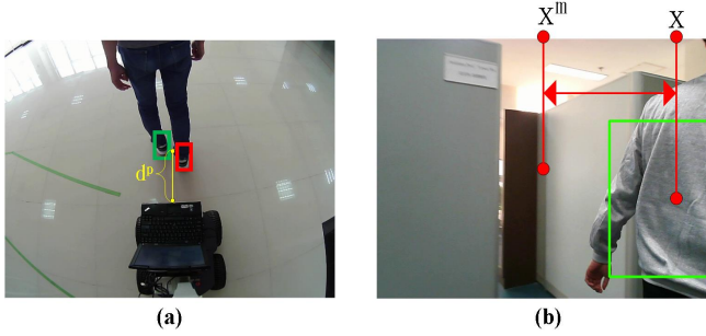
Fig. 4. (a) The distance d^P between the robot and the followed person can be calculated based on the feet tracking result. (b) The orientation information can be obtained based on the upper body tracking result.
